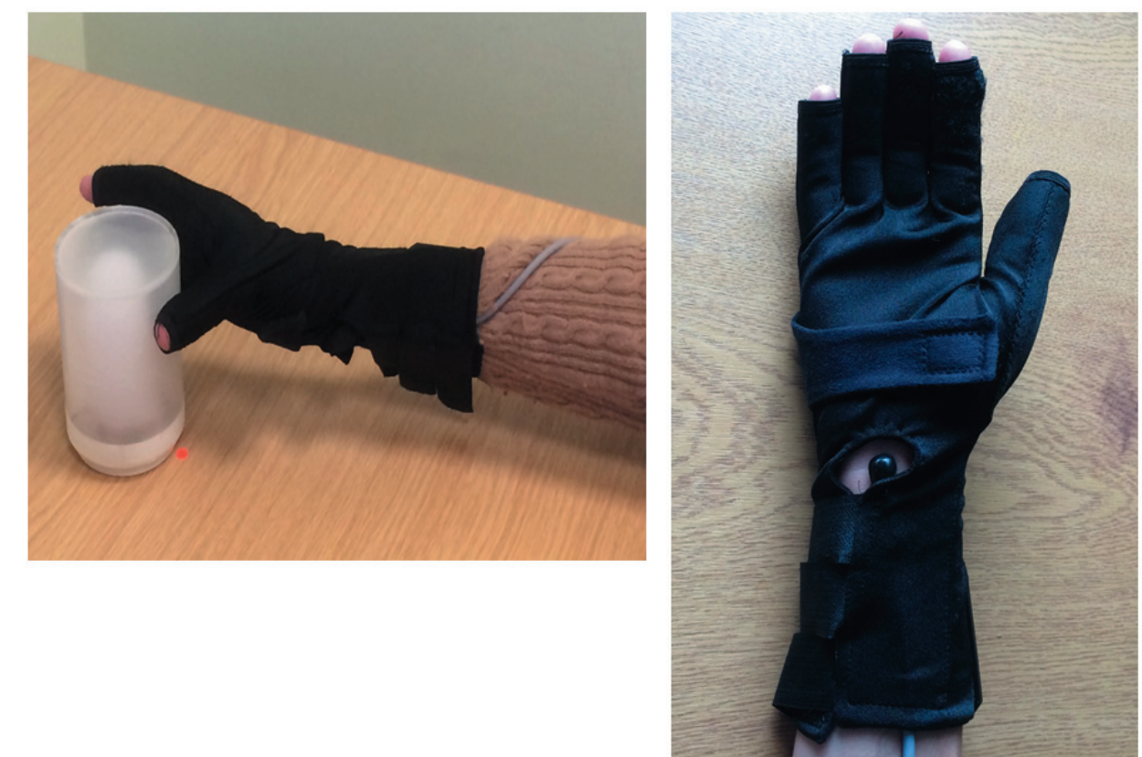
Figure 2: The data gloves contain embedded movement sensors
