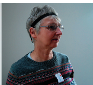
Figure 2: Movement sensors are easily attached using Velcro straps and may be worn under or over clothing
